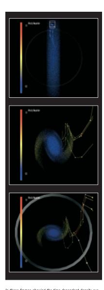
In these frames showing the time-dependent density evolution of an intense beam, the high density region is the beam core. Selected particles of interest, depending on the physical problem under study, are shown as streamlines. In this case, the streamlines correspond to halo particles in a very low density region far from the core. The spiral arms show the result of the beam's being injected improperly into the accelerator, which in this case is a separated sector cyclotron.
